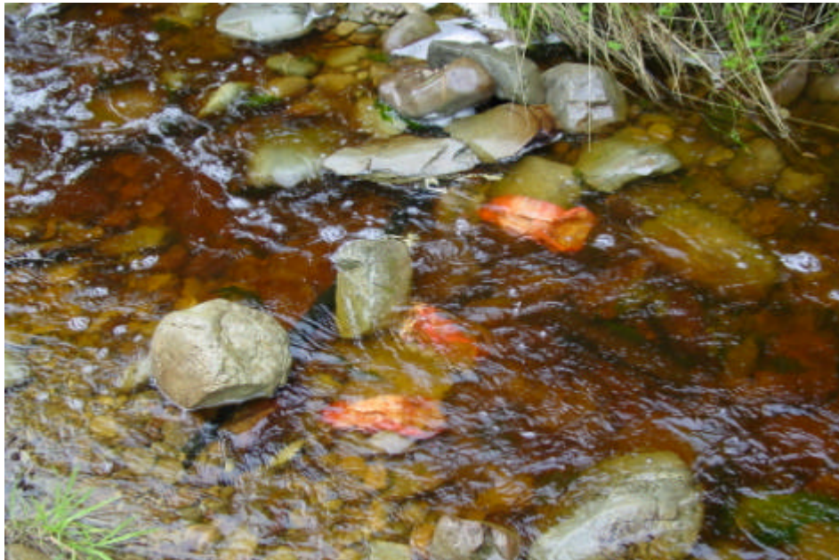
Figure 5: Photo of the 1080 baits placed in Deadhorse Trib. Equal numbers of baits were placed in coarse mesh bags, which were placed at even intervals across the stream to ensure complete mixing of any plume of 1080 compound that would leach from the baits.
